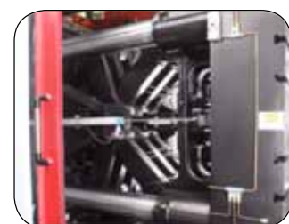
The 5-point double toggle provides short locking time and high opening force.
