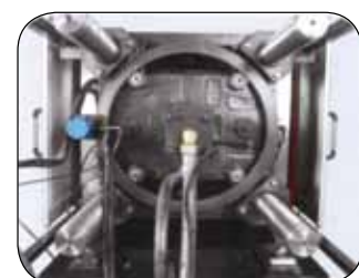
Automatic mould height adjustment ensure the time and cost saving during the mould changing.
