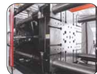
Mould platens have been designed using FINITE ELEMENT ANALYSIS for optimum rigidity.
